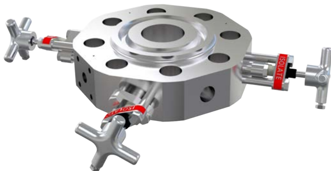
Through bore, multi outlet, MONOFLANGE manifold. Branch 1, double block – OS&Y Isolate-HP outlet-OS&Y Isolate-HP outlet. Branch 2, single block – OS&Y Isolate-HP outlet
