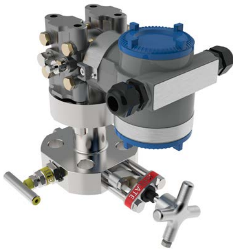
Close-Coupled Double Block and Bleed MONOFLANGE with IEC 61518 TYPE B Outlet connection (not differential) Horizontal Mount. Primary OSY isolate, standard needle valve in secondary isolate and vent, with 1/4" NPT plugged vent outlet.
